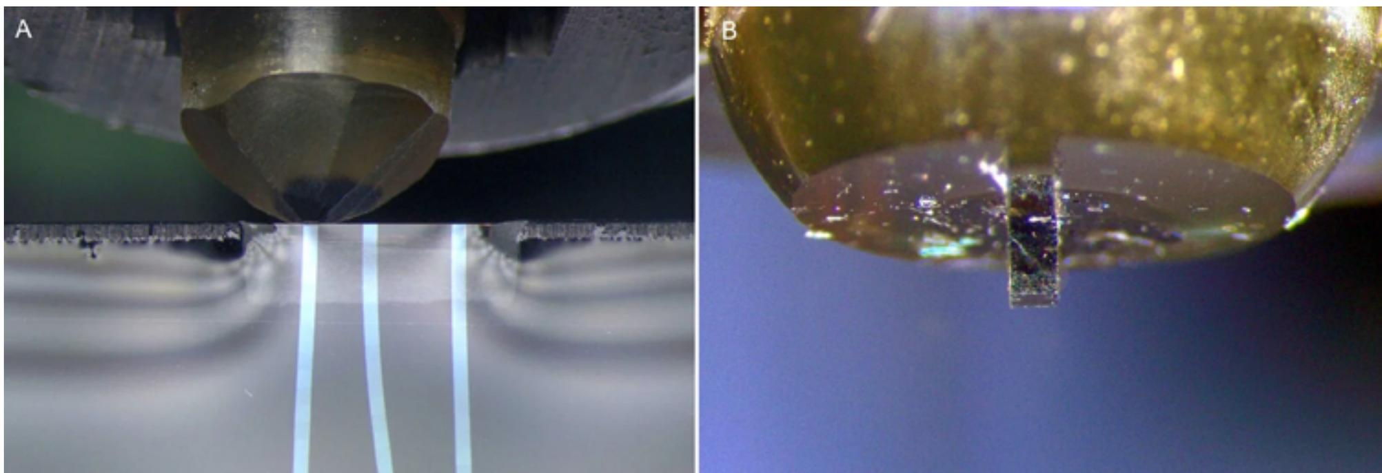
Figure 24: Features of the ARTOS 3D solution which lead to a more efficient workflow include: A) automated serial sectioning with seamless transition to the following ribbon without thickness variation and B) auto-trimmed block face of a resin-embedded specimen (size 0.5 x 0.5 x 1 mm).
